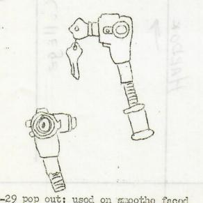
1928-29 pop out; used on smoothe faced instument panel (with oval speedometer, up to June 1930 and until an assembly plant had used up it's stock.
