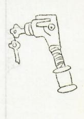
1930-31 Model A Ford orginal pop out. Used with lined instrument panel, and round speedometers. Notice front view. There is no (fat) right hand extension of the pop metal type housing. GEO. + DARIEUE STAID
